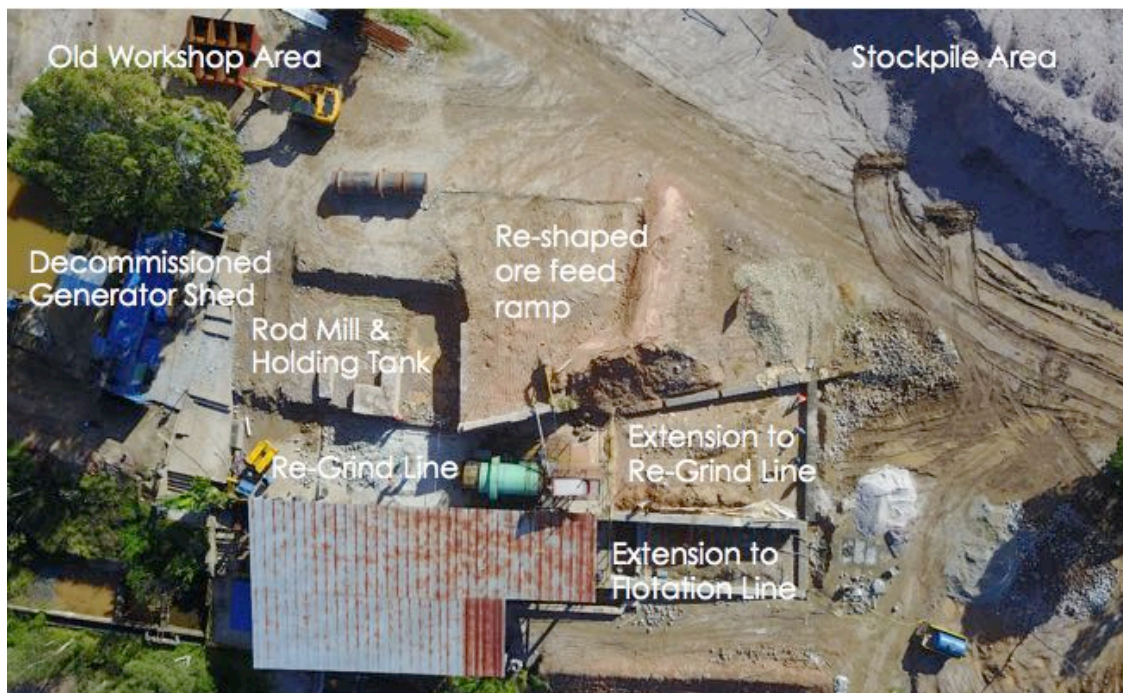
Figure 1: Process Plant with civil work underway to extend foundations and reconfigure equipment layout.
