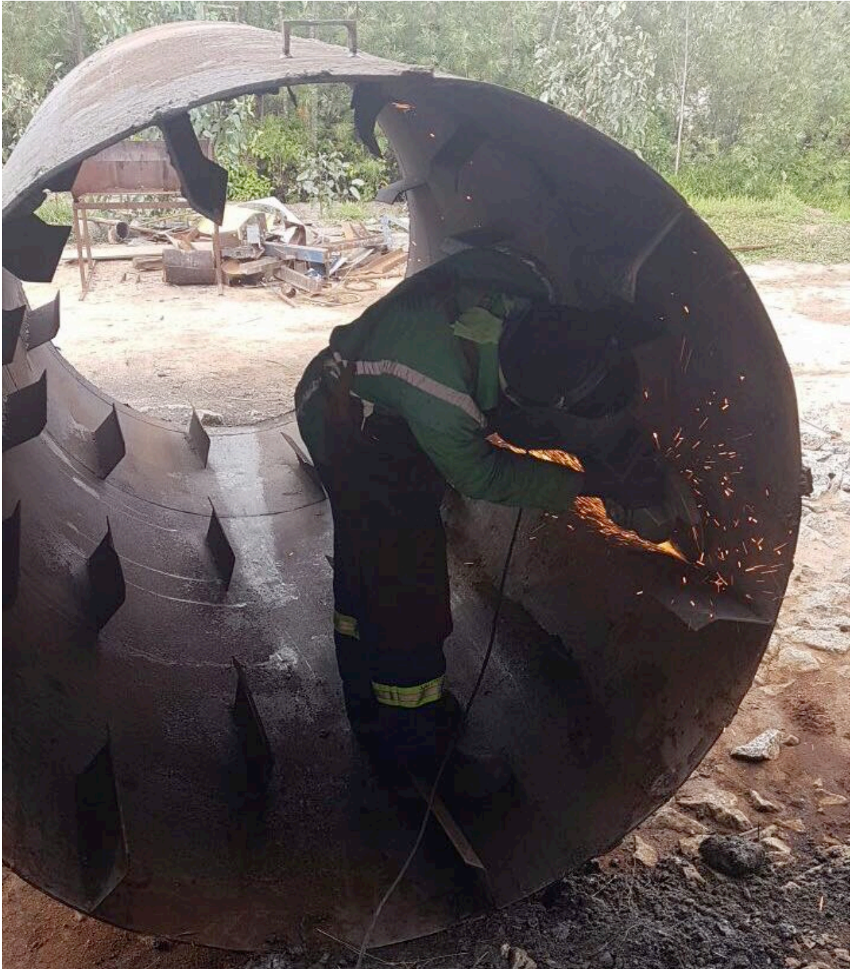
Figure 7: Refurbishment of decommissioned rotary dryer drum to become the new Spinners feed bin.
