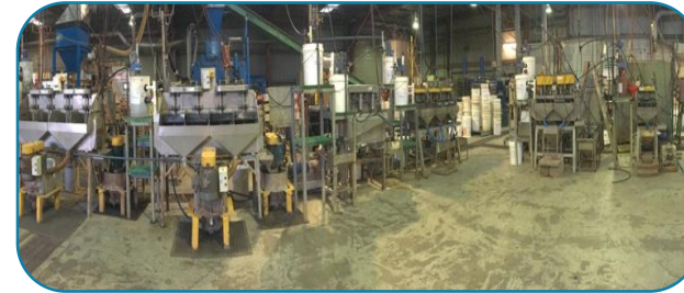
Flotation Pilot Plant Operation at ALS, Perth
