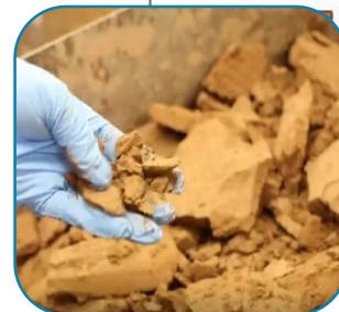
Final flotation concentrate to hydrometallurgy pilot
