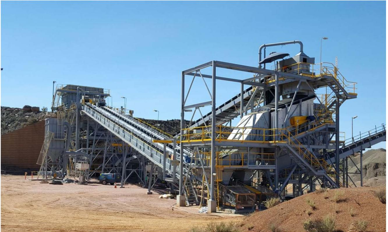
Refurbished Crushing Circuit with new triple deck screen (foreground) and upgraded feed bin (background).
