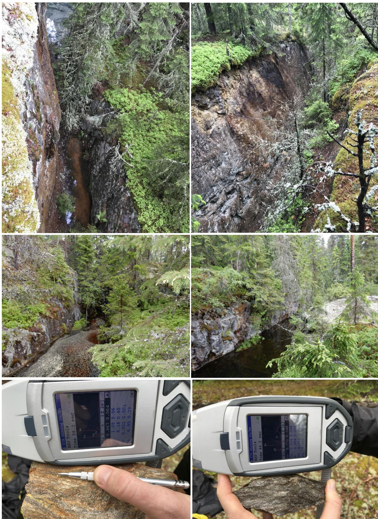
Figure 1 | Field Photographs: Showing extent of historic workings at Skuterud and spot handheld XRF analysis of disseminated sulphide mineralisation
