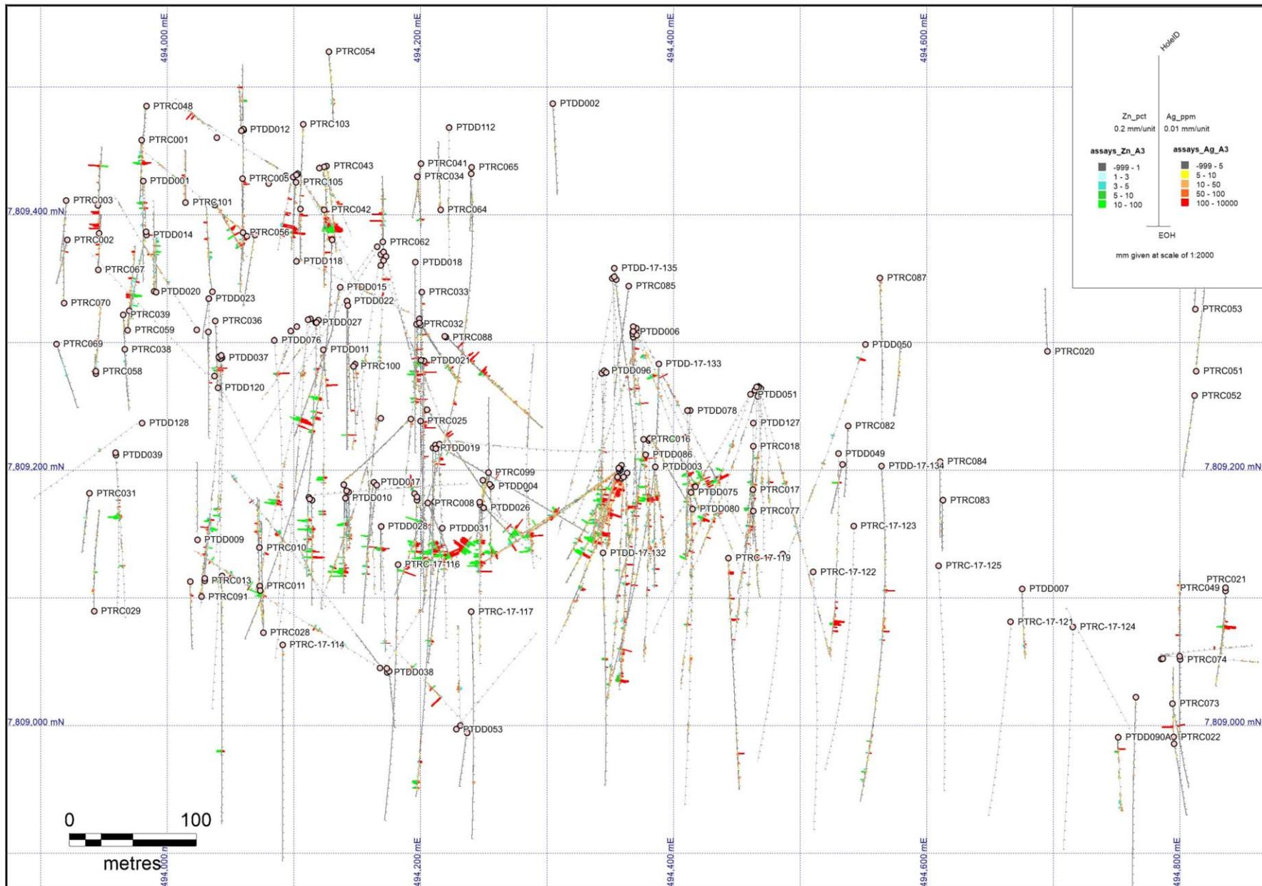
**Figure 4.** Patricia drill holes used for the resource estimate with downhole zinc and silver geochemistry in plan view.
