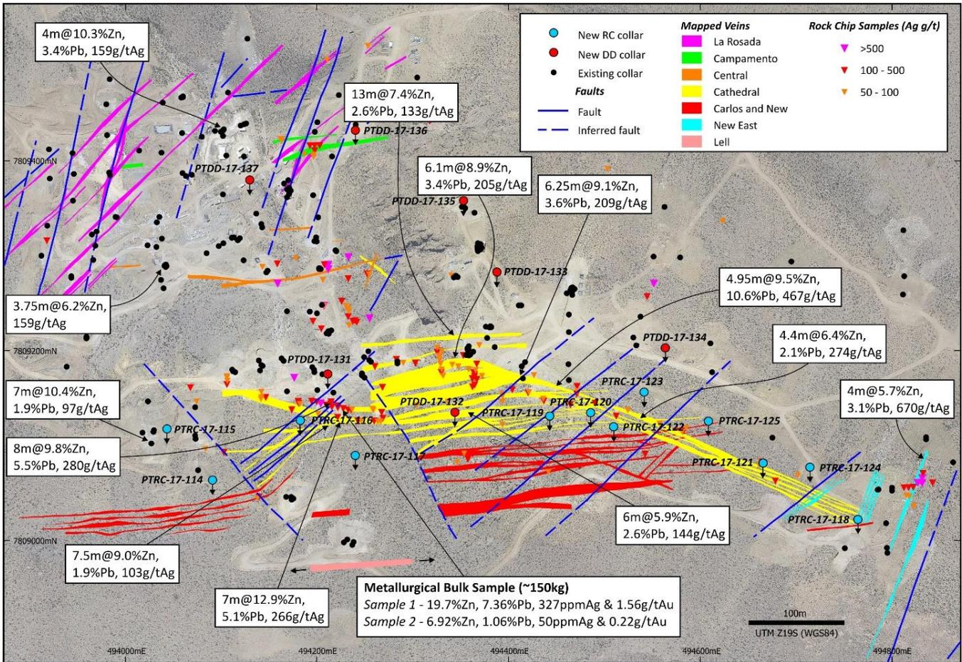
**Figure 3.** Plan showing the mapped zinc-silver-lead veins at Patricia and the location of Golden Rim's recent diamond drilling (red circles) and RC drilling (blue circles).
