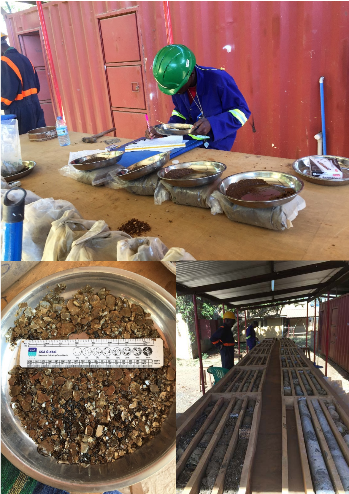
Fig 6. AC logging (Top), AC chips rich in vermiculite flakes (Bottom Left), DC logging (Bottom Right)
