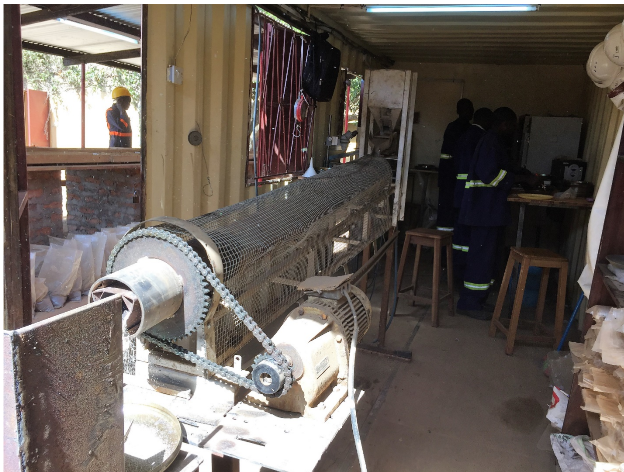
Fig 7. Rotary Muffler/exfoliator used for Vermiculite analysis
