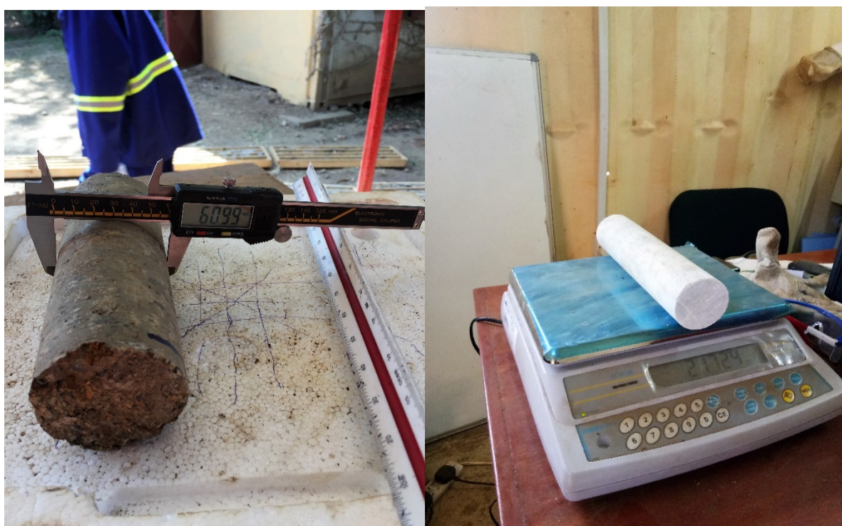
Fig 9. Caliper Bulk density method
