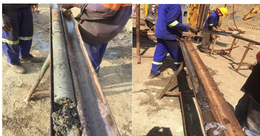
Fig 3. Core removal from split inner tube
