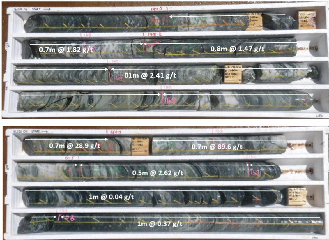
**Figure 2: Diamond Drill Core from 16LCDD004**
