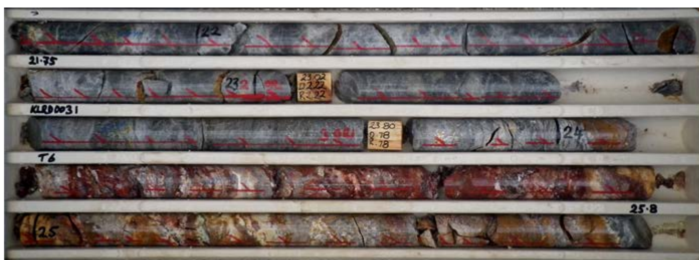
Photo: KLRD0031 intense silicification and local feldspar alteration of andesitic rock in the hanging-wall of the main Koala lode vein. Banded, oxidised quartz-limonite vein from 24m returned 2m @ 85 g/t Au representing a small pillar of remnant ore near the old main shaft.
