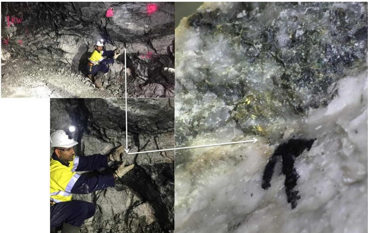
Photo 2: Visible gold in the Golden Age 980 ore drive
