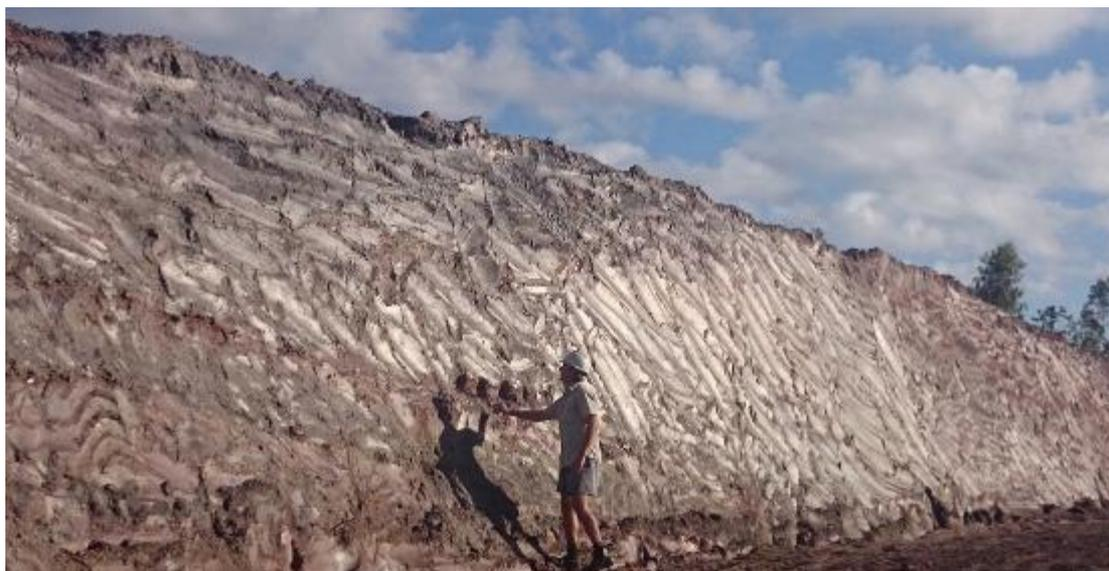
Loharano mining bench with highly reflective graphite mineralisation near to surface.
