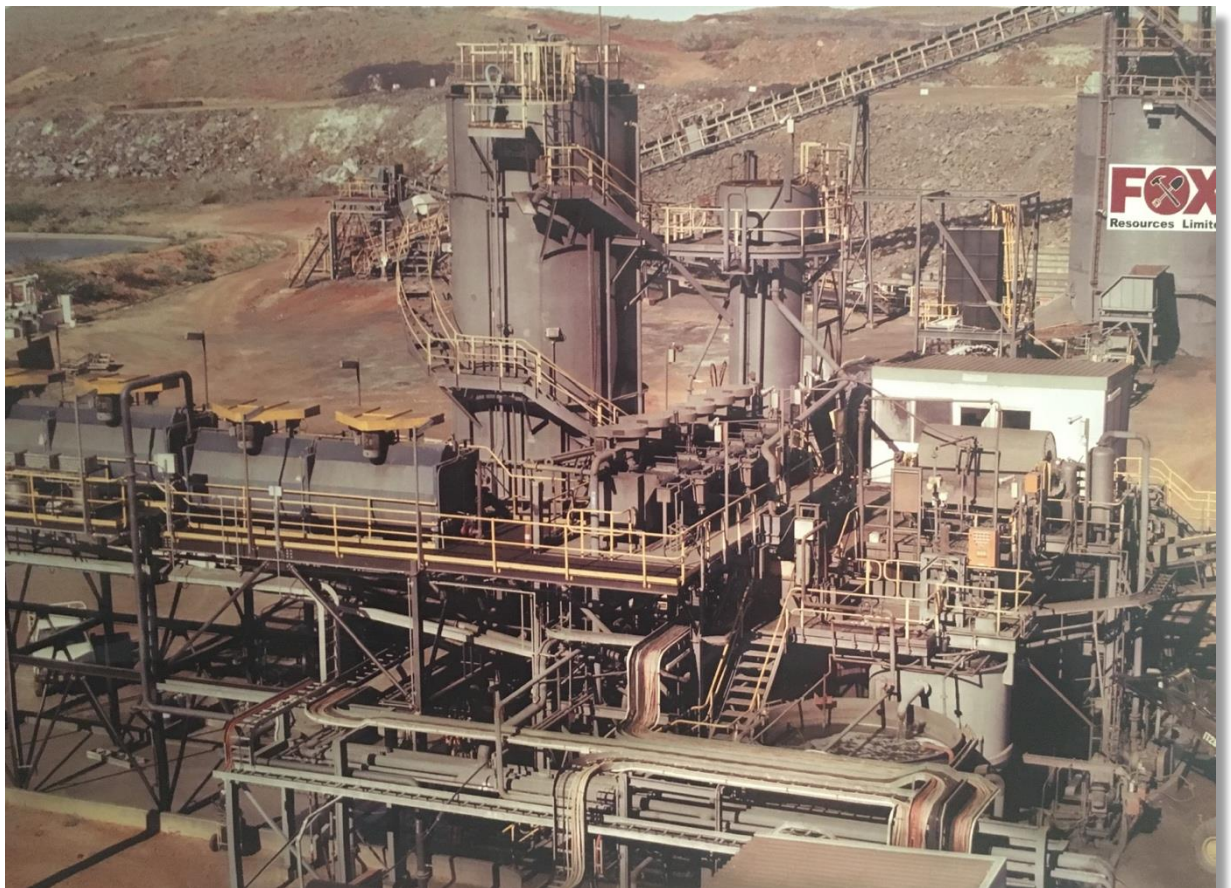
Figure 6: AGIP Radio Hill Nickel/Copper Operations (Fox 100%) – Radio Hill 425,000 tpa Treatment Plant and floatation circuits.
