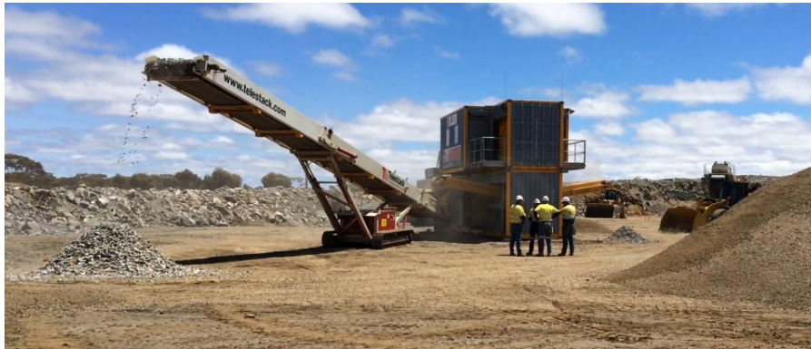
Ore sorter in operation at the Flying Fox mine-ore-pad
