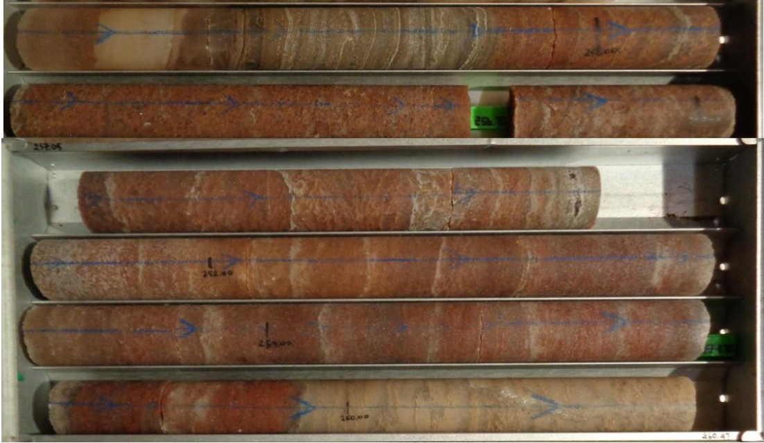
Figure 1. The Hangingwall seam sylvinite in EK_49 (orange-pink colour). 4.04 metres grading 58.9% KCl. Rock-salt above and below the seam is included in the photograph
