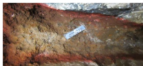
Figure 3 LEFT: Photo of samples IM-001309-11-12. Sample IM-001311 contains 33.91% Zn, 6.81% Pb and 4.5g/t Ag . INSERT BELOW: Photo of the mineralised vein at the Wari mine working at La Elegida 1. Sample IM-001078 contains 33.76% Zn, 169g/t Ag and 17.33% Pb .
