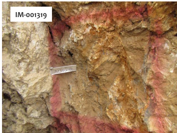
Figure 4 ABOVE LEFT: Photo of sample IM-001319. Sample IM-001319 contains 32.86% Zn, 0.45% Pb and 98.6g/t Ag . ABOVE RIGHT: Close-up of the breccia structure subject of sampling. Dolomitised limestone clasts (orange brown rock fragments) can be seen with a gossanous and galena-bearing matrix.
