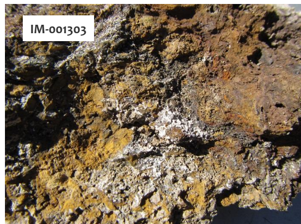
Figure 5 RIGHT: Outcrop photo showing detail of Sample IM-001303. The highly weathered and leached nature of the sample is evident. It is highly gossanous which is an indication of original high sulphide content. It contains 16% iron (Fe).
