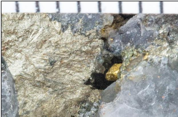
Visible free gold next to fresh sulphide (arsenopyrite) in quartz-carbonate veining from 263.80m down hole TGGRCDD110. Scale bar at top is in millimetres. ASX announcements dated 15 November and 12 December 2017 present full details.
