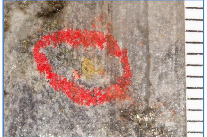
Figure 13. Free gold and sulphide at 264.80m.
