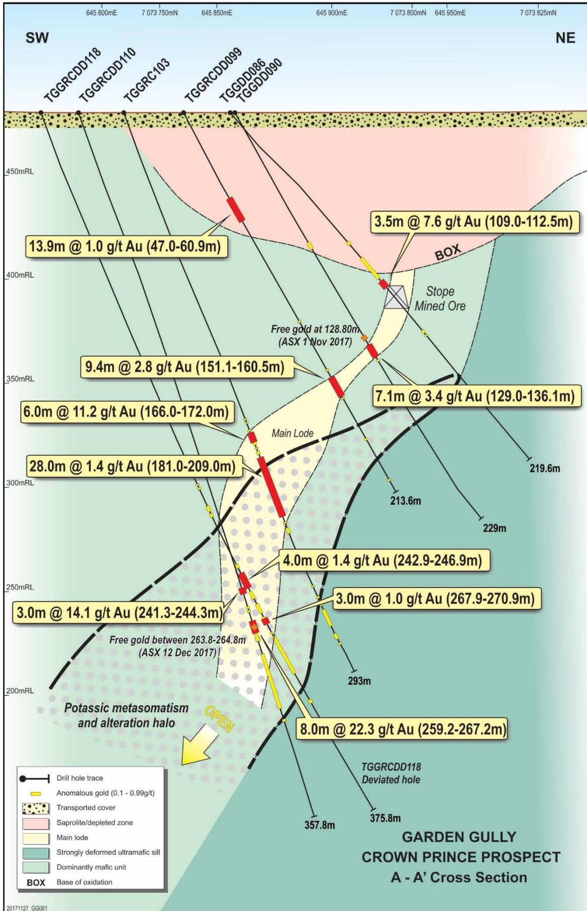
Figure 4. Crown Prince Prospect. Cross section A-A' through the Main Lode, looking north-westerly.
