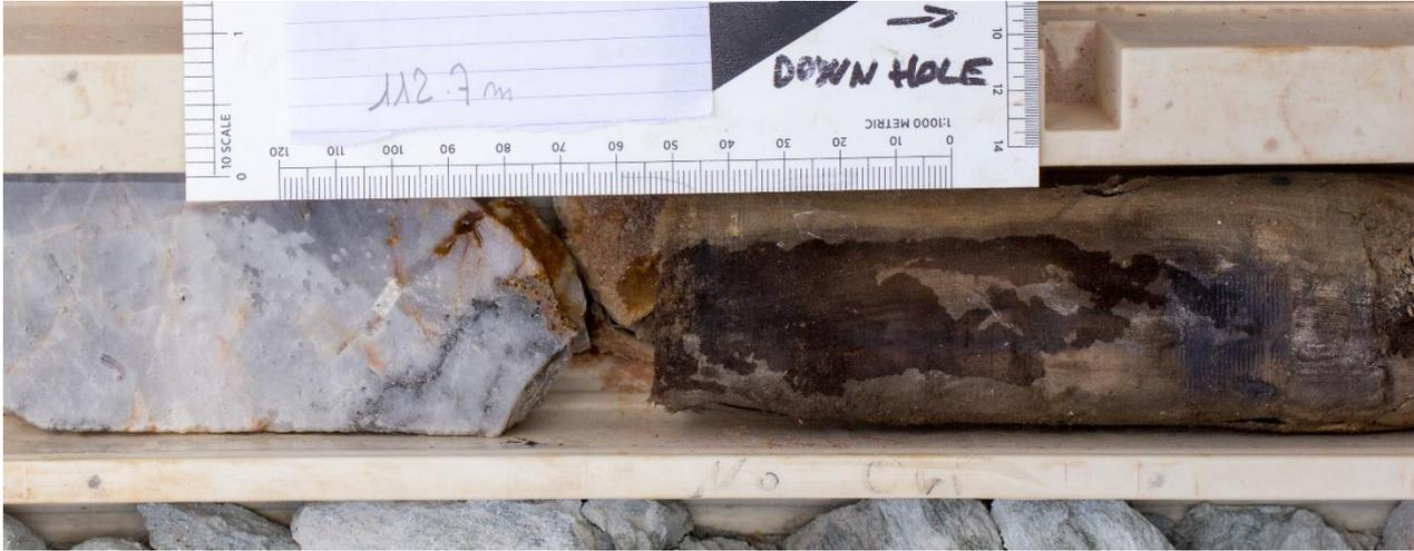
Figure 5. Crown Prince: wooden core from unmapped old stopes at 112.7m in TGGDD086.
