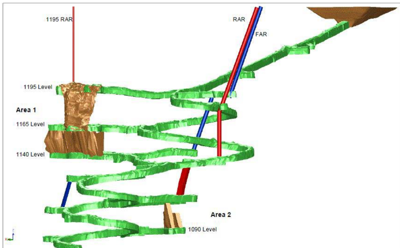
Figure 4: Underground workings at the 309 Deposit (decline and level development –green, stopes –brown) with the decline extending to approximately 170 m below surface (surface RL is approximately 1250 m.). Significant development is in place adjacent to the Area 2 mineralisation, however very little of this deposit was extracted.
