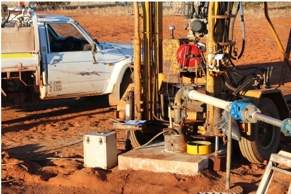
Figure 2. Karlawinda Gold Project – Borefield Pump Testing
