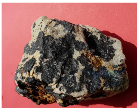
Figure 1: The cobalt oxide-hydroxide that occurs as black spots or dendritic growth in dolomitic/limestone rocks
