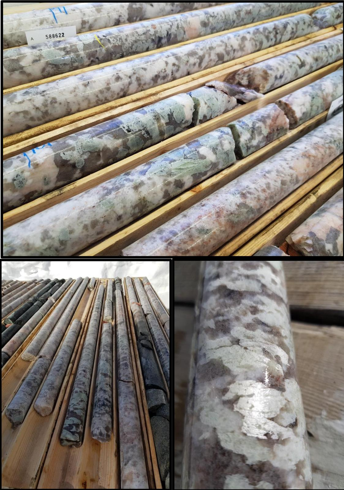
**Figure 2.** Three images of the drill core obtained from drill hole SA-18-07, Note large pale green to whitish coarse tabular spodumene crystals with quartz and feldspar.
