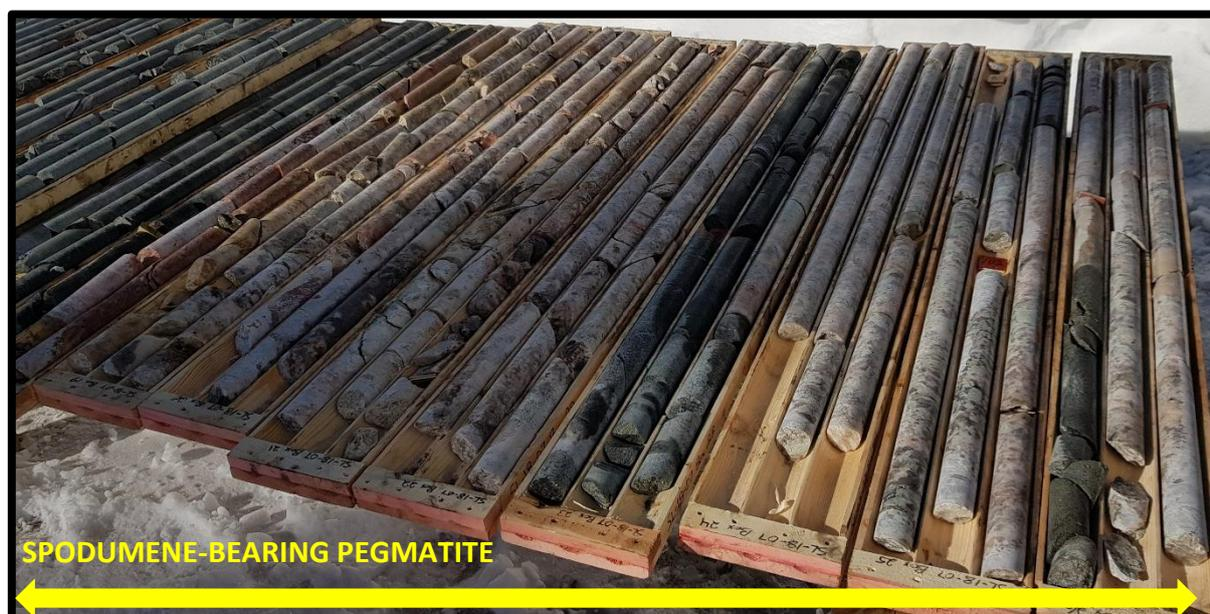
**Figure 1.** Drill core obtained from drill hole SA-18-07 (from approx. 55m to 109m) showing the intersection of high-quality spodumene-bearing pegmatite (the lighter coloured material in the photo is the Pegmatite, whilst the darker material is Mafic Volcanic).
