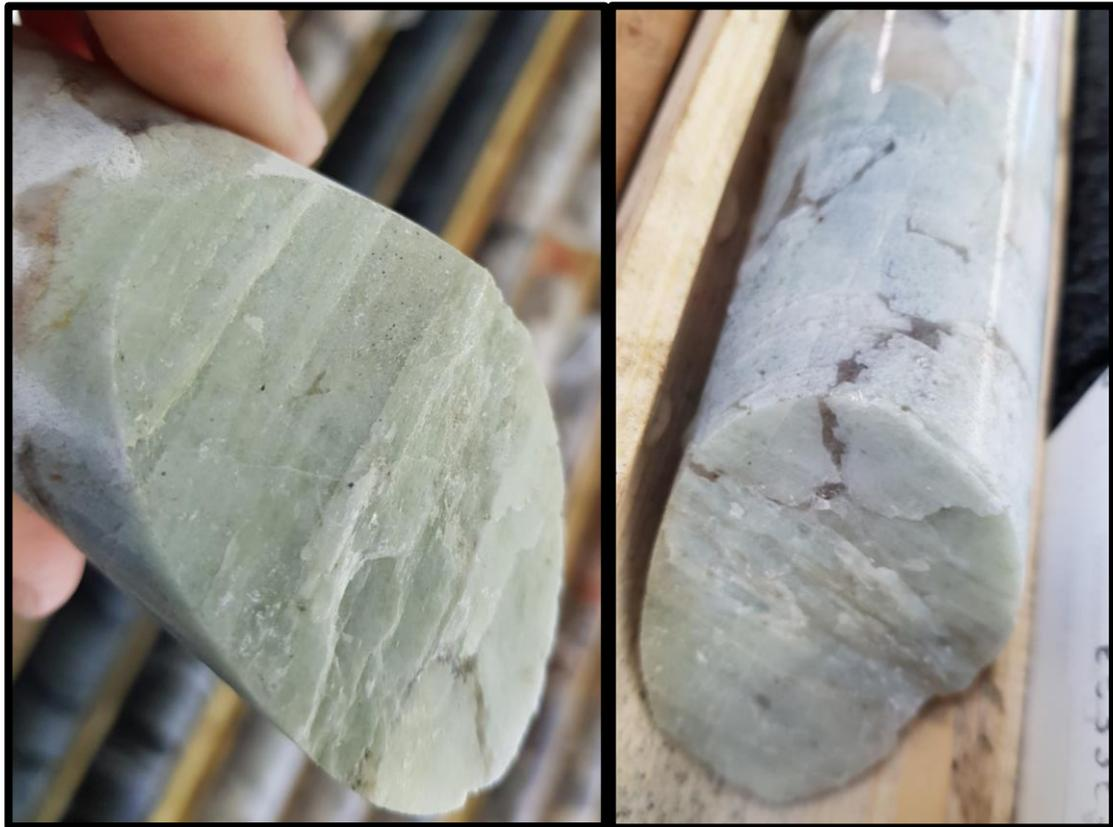
Figure 3. Drill core images obtained from drill hole SA-18-07 show very large high quality spodumene crystals.
