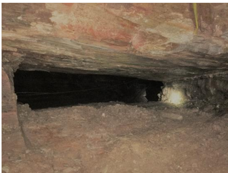
Stope trial – stope width of 0.75m achieved
