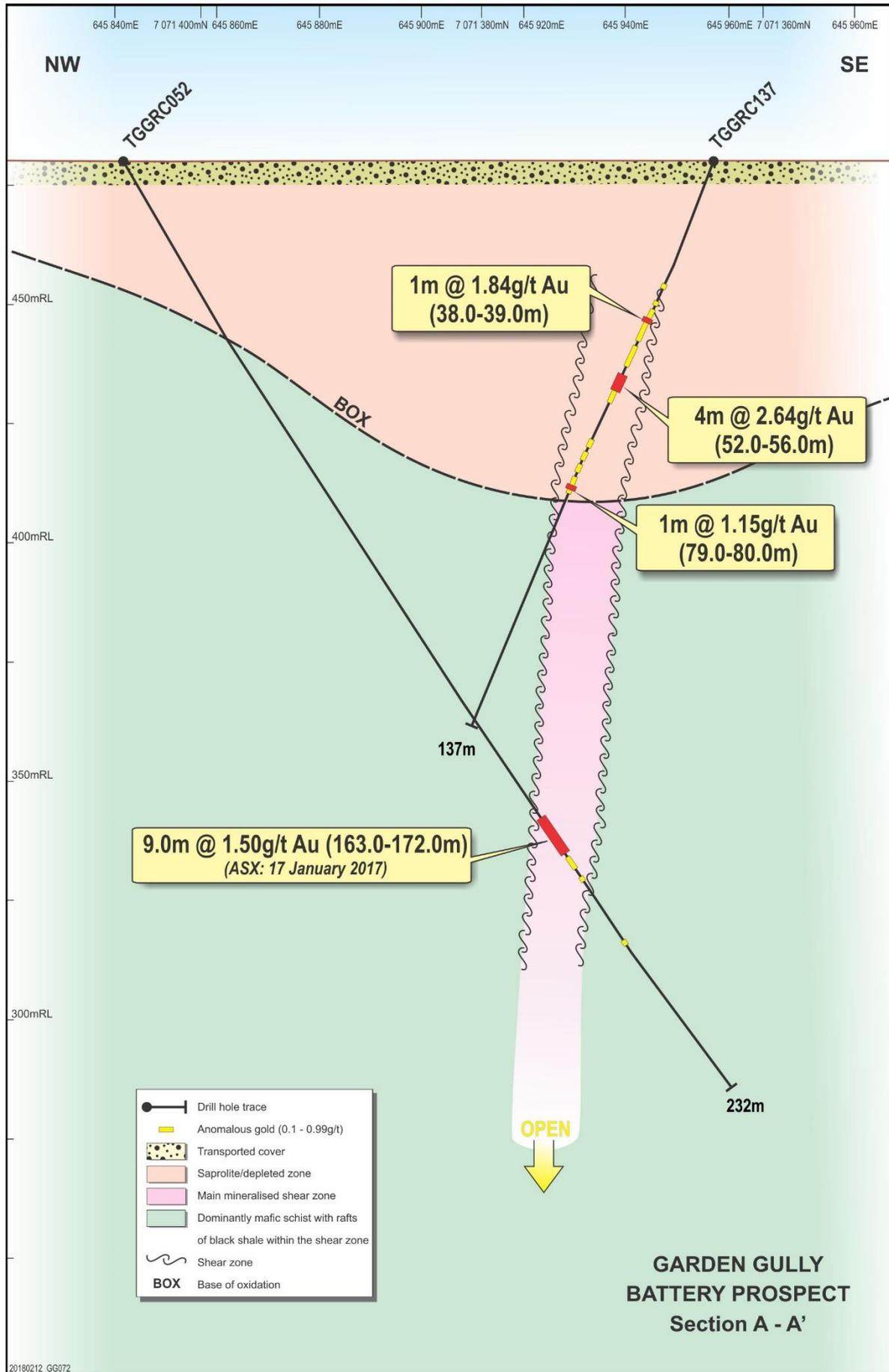
Figure 8. Cross section A-A' through the northern part of the Battery mineralised shear (refer Figure 4).
