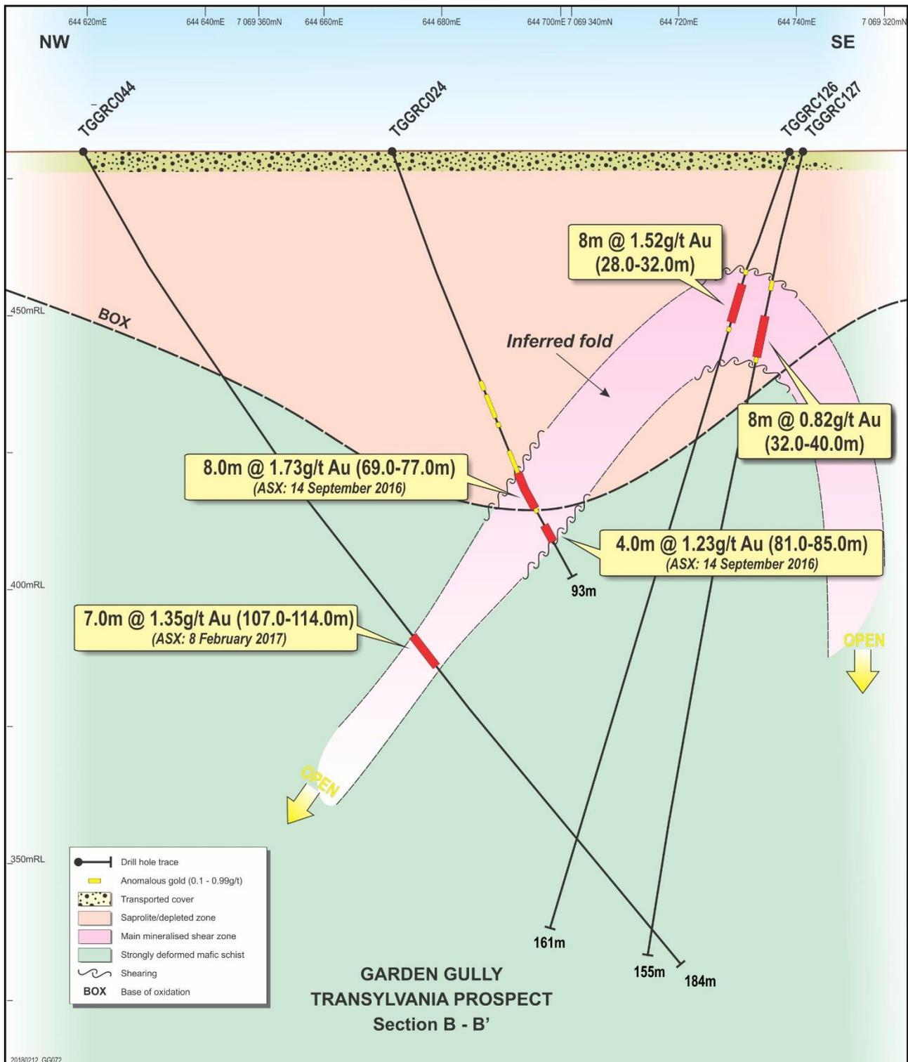
Figure 7. Cross section B-B' through the northern part of the Transylvania mineralised zone (refer Figure 4).
