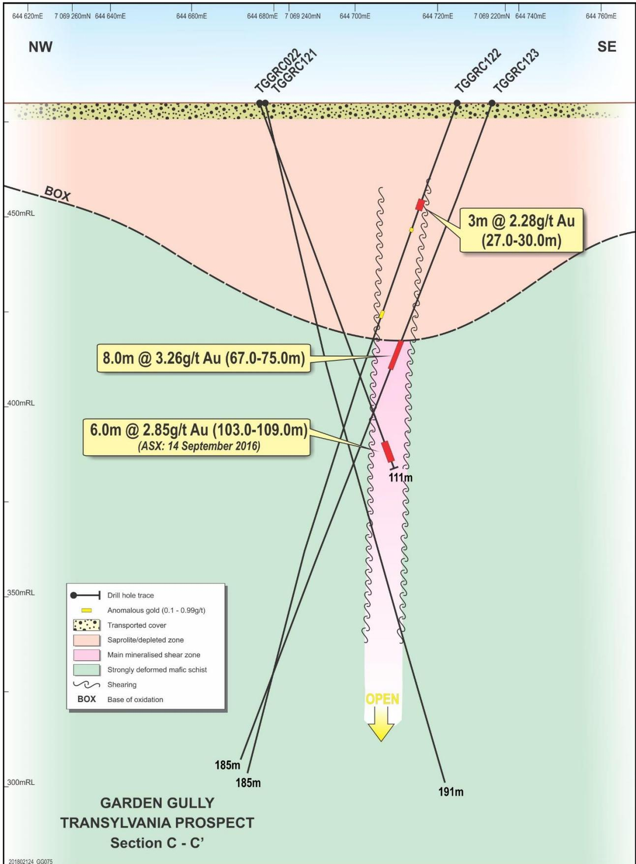
Figure 6. Cross section C-C' through the southern part of the Transylvania mineralised zone (refer Figure 4).
