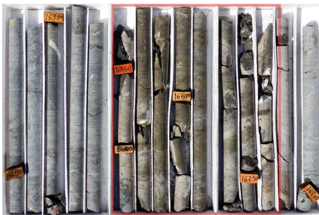
Figure 6. Massive sulphide mineralisation intersected in LV5040 drill hole from LV5040 core with massive sulphides zone from 164.15 to 168.50 meters hosted in Juarez Limestone. Sphalerite with pyrite patches at hanging all contact. Another 1m zone from 176.05m occurs on the footwall contact
