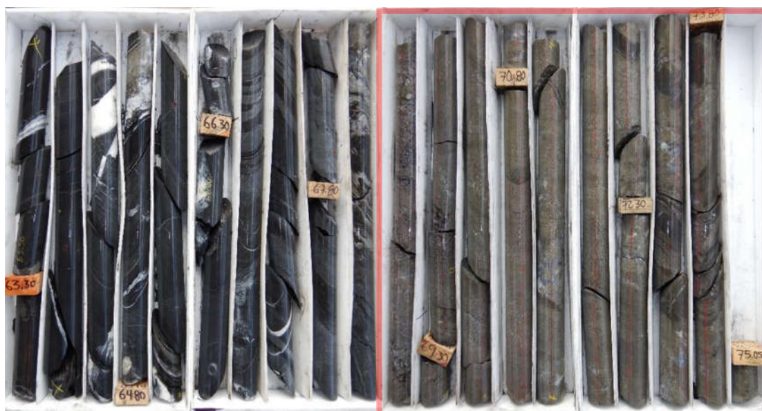
Figure 3. Massive sulphide mineralisation intersected in LV5039 drill hole from 68.25 to 73.85 metres (5.6m); very fine-grained sphalerite overprinted by yellow to reddish sphalerite and minor galena.
