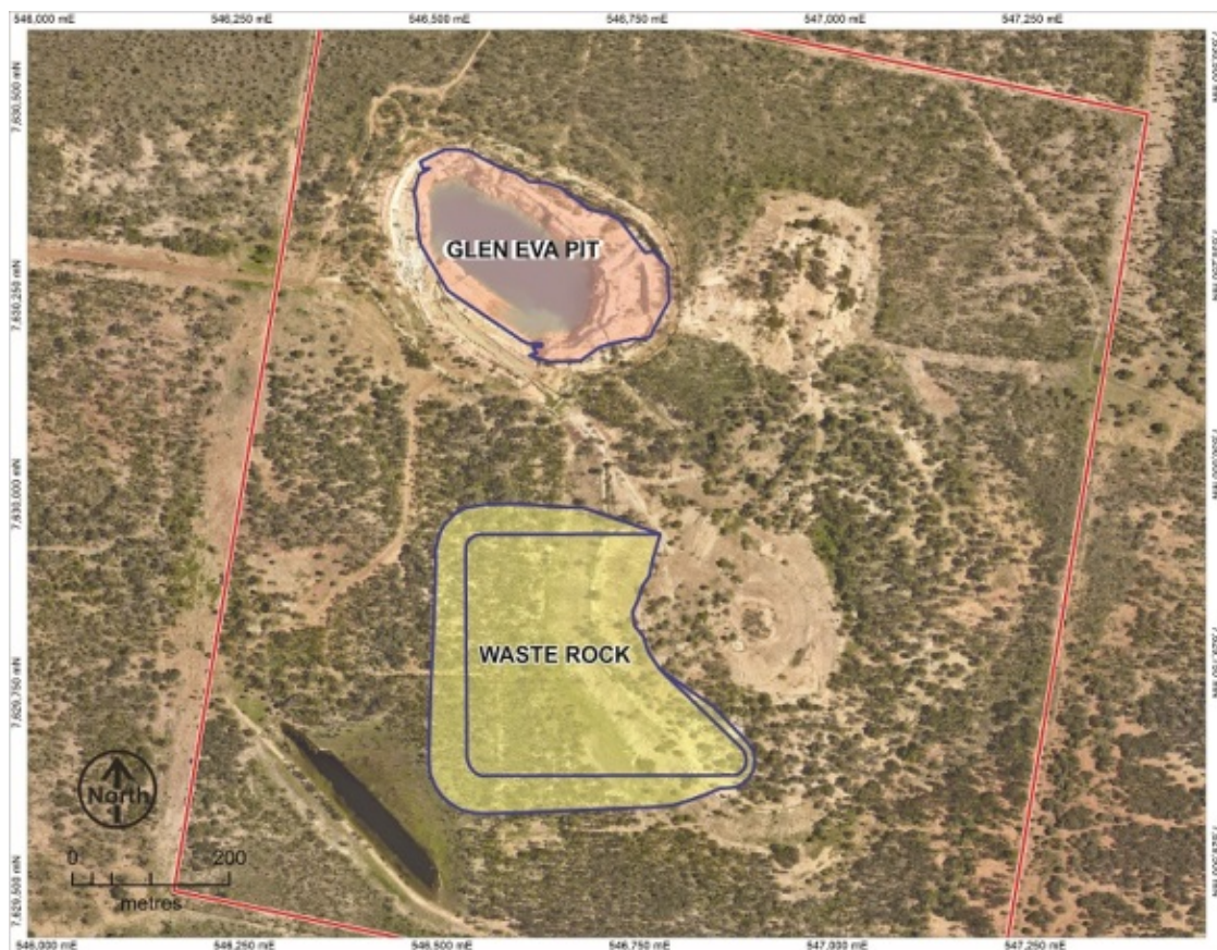
Glen Eva Final Pit Design mines the previous pit which ceased in 1996 and mine layout.
