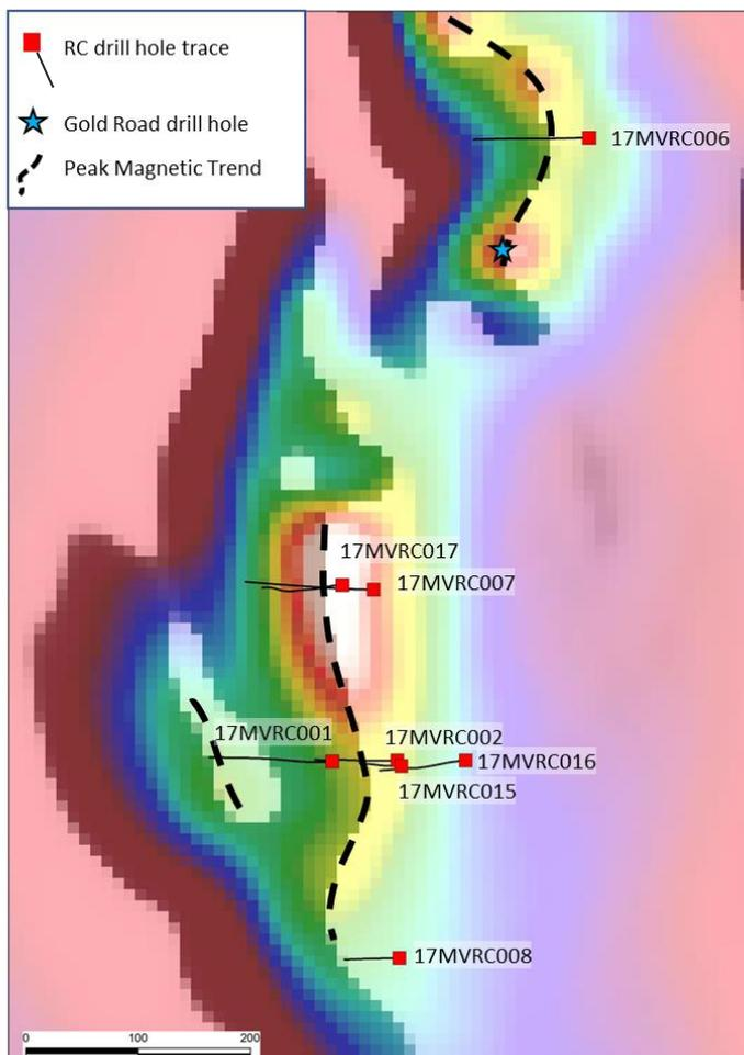
**Figure 2.** Central mineralised zone showing magnetic trend and drill hole traces
