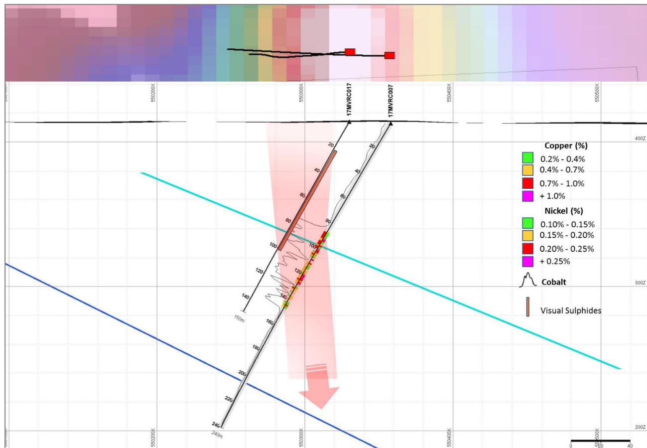
Figure 4. X-Section 6887660mN with modelled EM conductor plates (TMI-1VD magnetic image top)
