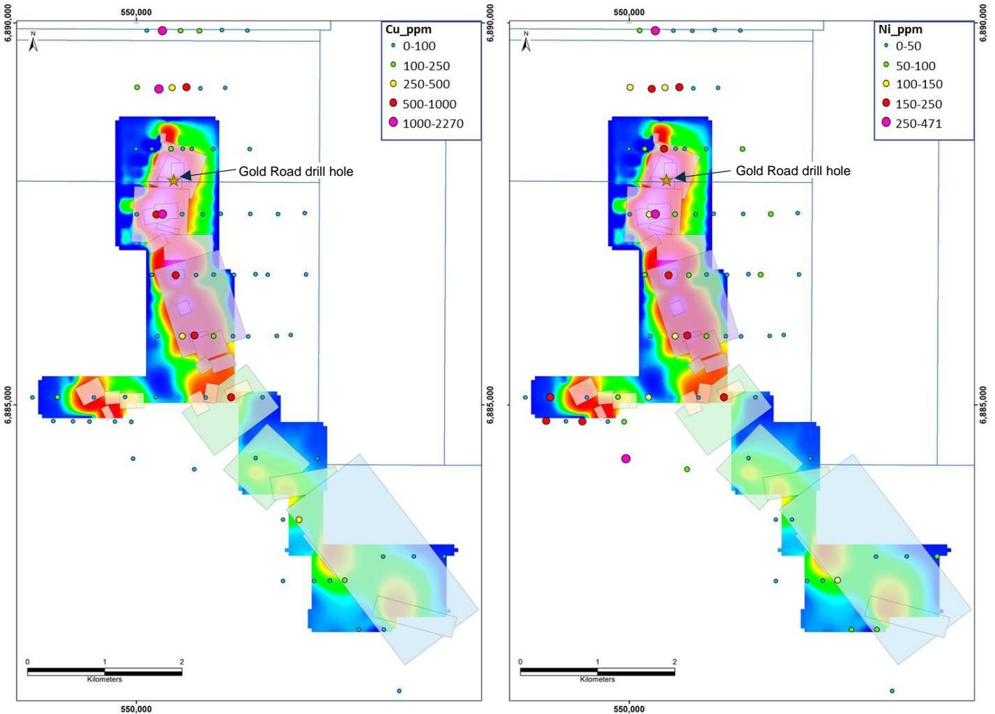
**Figure 8.** End of hole copper (LHS) and nickel (RHS) grades shown over Channel 30 EM response. Note the EM survey does not cover the northern extension of the Cu-Ni anomaly
