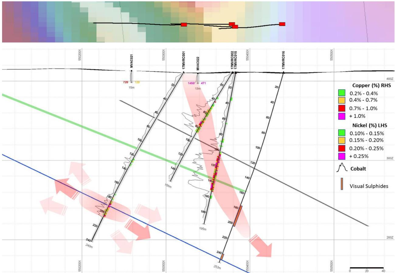
Figure 3. X-Section 6887500mN with modelled EM conductor plates (TMI-1VD magnetic image top)
