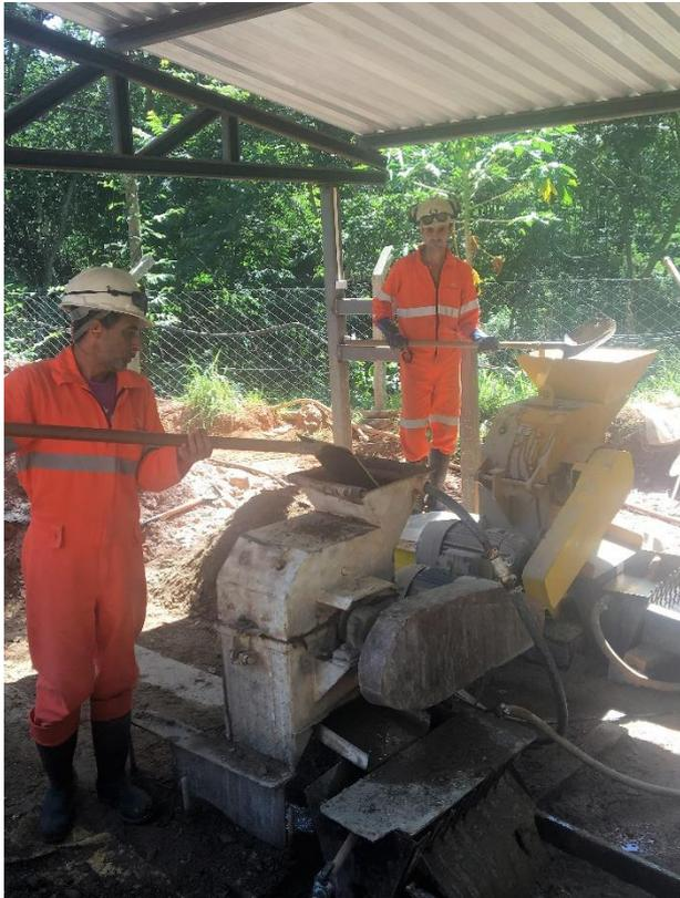
Figure 1; Two hammer mills operating
