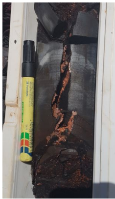
FIGURE 5: NATIVE COPPER INTERSECTED IN HOLE 17MCHMET004 AT 82.8M
