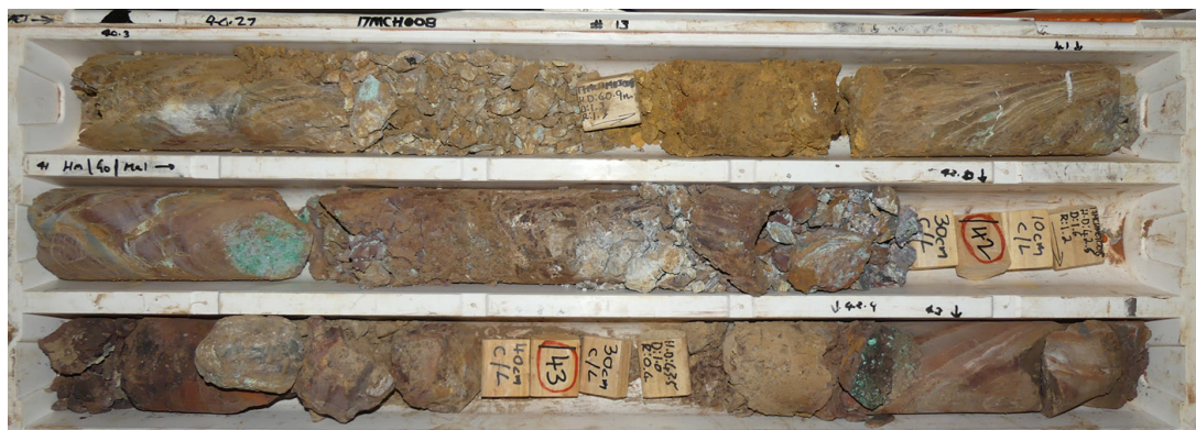
FIGURE 3: INTERVAL OF MALACHITE AND FE-OXIDE MINERALISATION IN HOLE 17MCHMET008 AT 3.6% CU (PRELIMINARY DATA FROM TRUESCAN XRF)
