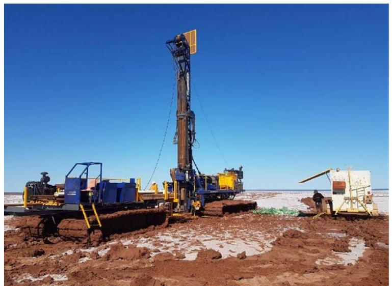
**Figure 4** Drill rig completing water bore to support diamond drilling operations
