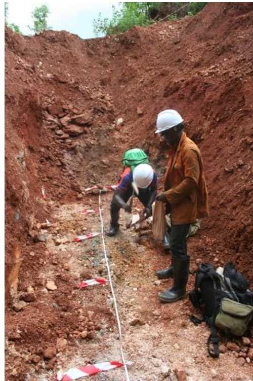
Figures 1 and 2. Commencement of Trench 003 and channel sampling exposed pegmatite at base of Trench 001.
