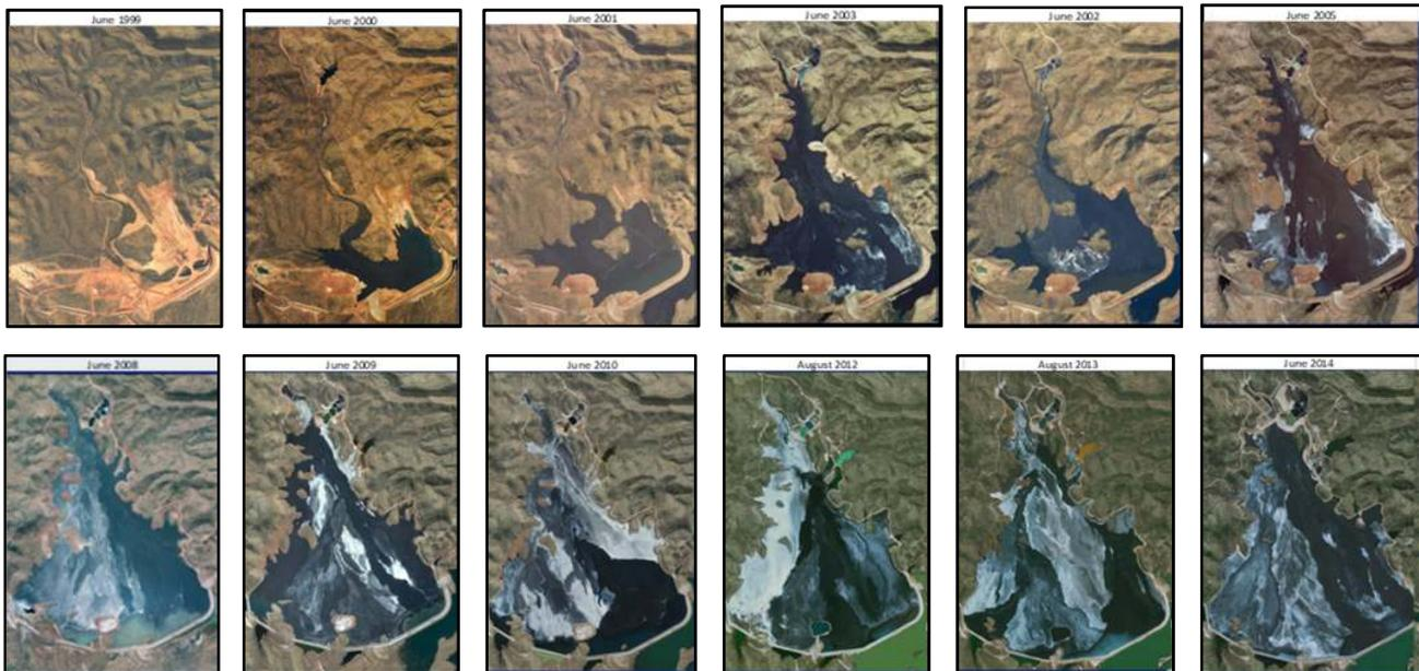
**Figure 6: Evolution of the Century Tailings Deposit (1999 to 2014)**
