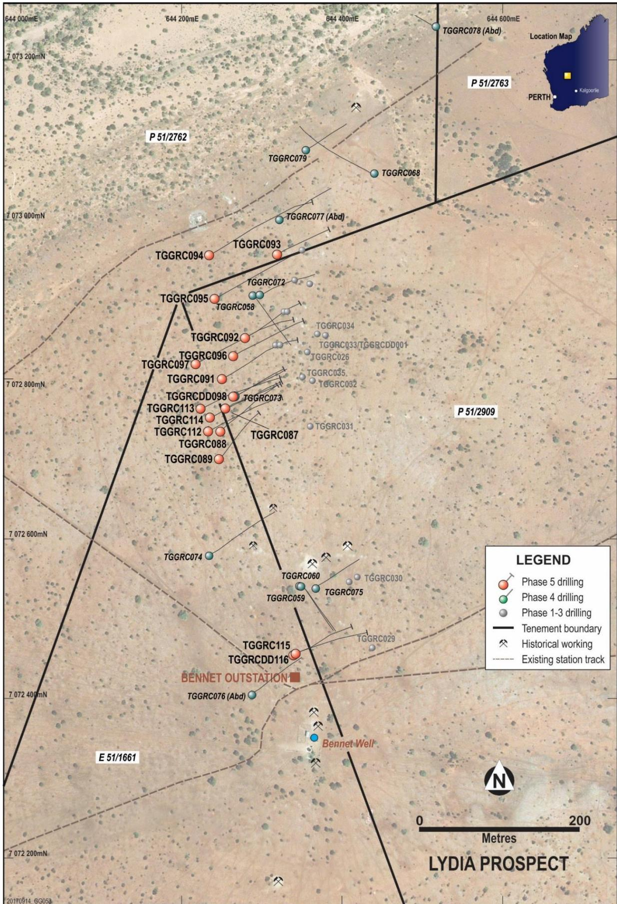
Figure 4. Drill collar locations and drillhole traces from the holes drilled at Lydia Prospect in the current Garden Gully phase 5 drilling programme.
