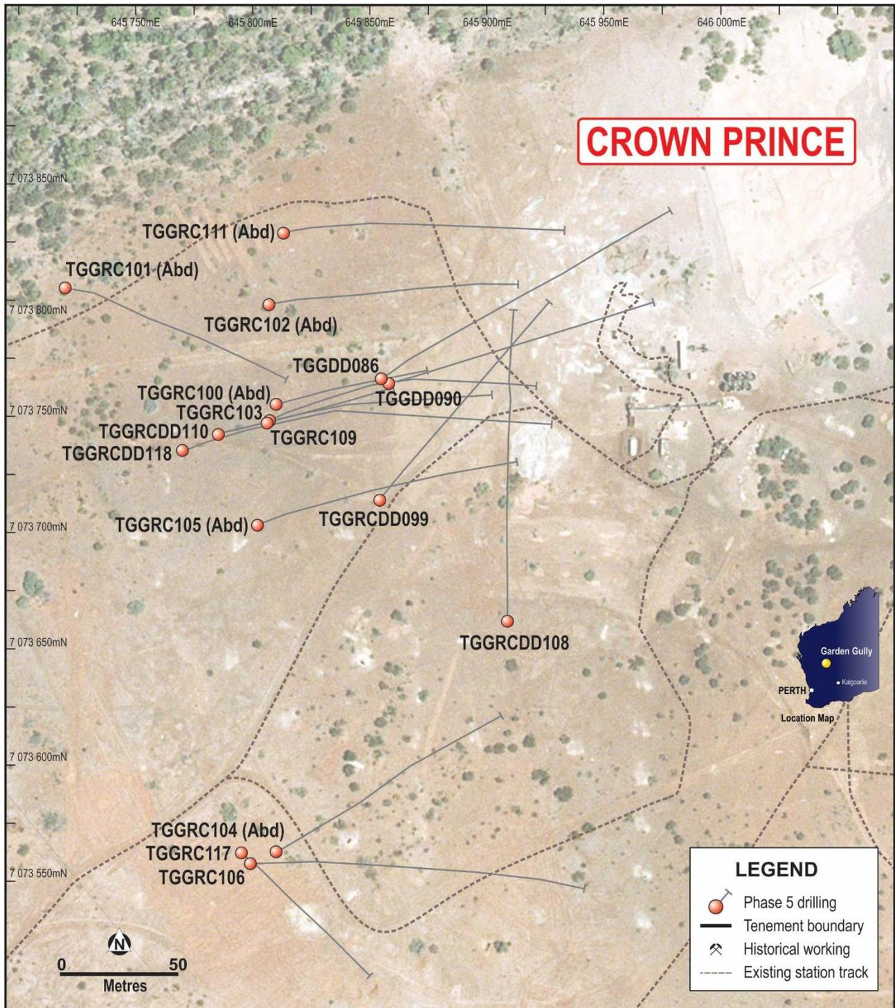
Figure 3. Drill collar locations and drillhole traces from the holes drilled at Crown Prince in the current Garden Gully phase 5 drilling programme.
