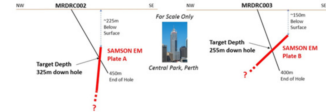
Figure 7. Section view of planned RC drill holes, MRDRC002 and 003, to target HP-MLTEM SAMSON conductive plate models A and B, Tyrrell's target area. Modelled conductive plates A and B on Lines 8B and 9B were interpreted to represent high conductance (4-6000 Siemens) bedrock features with at least 150m modelled depth extent down plunge.
