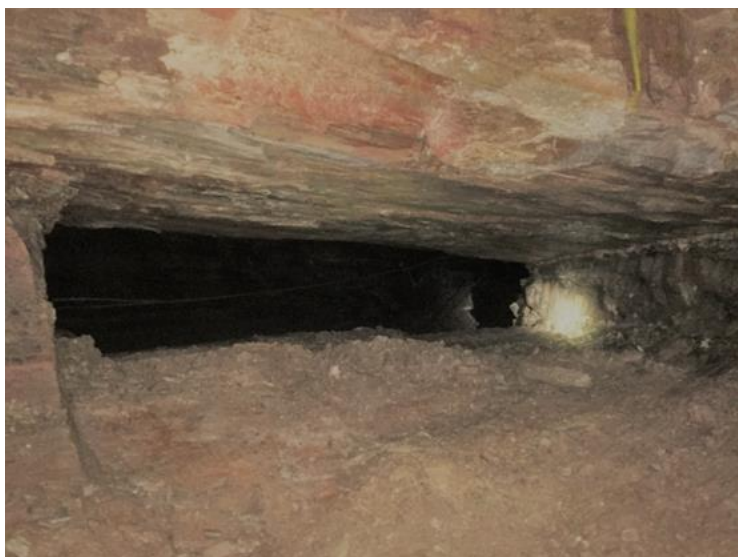
Image 1: L3C stope trial – stope width of 0.75m achieved
