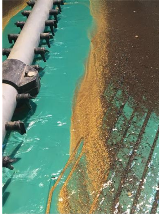
Image 2: Tabling of Concentrate from Mestre Decline
