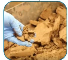
Final flotation concentrate to hydrometallurgy pilot
