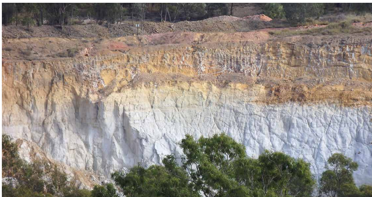
Koala open pit mined 1996. The softer, deeply weathered material is observed on the northern part of the deposit and is not expected to require blasting for excavation
