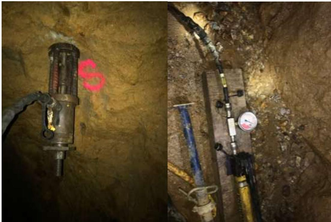
*Figure 3 - Rock bolt undergoing pull tests after installation. A hydraulic jack is attached to the anchor and load applied to the bolt. This tests the performance of the contact between the bolt, the resin and the ground being supported .*
