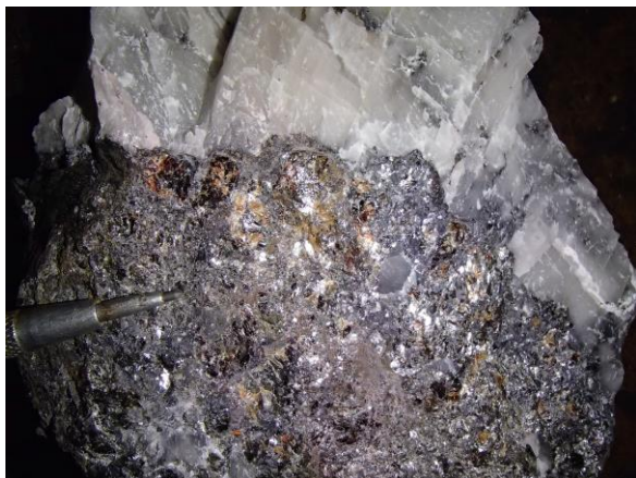
Figure 3. Photo of the massive sulphide from sample 38043, results are 28.8% Zn, 13.2% Pb, 41.4g/t Ag taken from wall exposure
