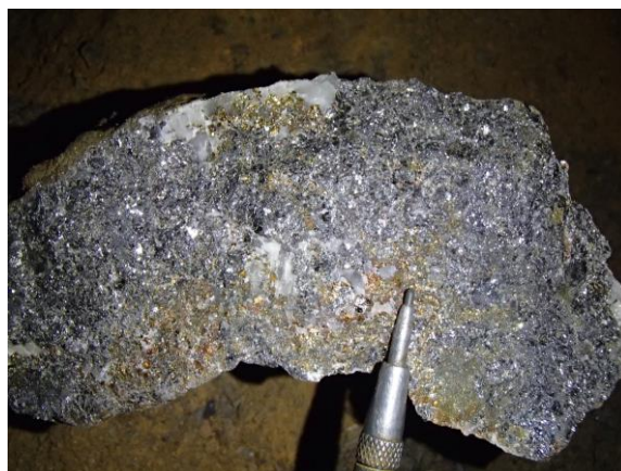
Figure 2. Sample 38040 runs 22.2% Zn, 3.55% Pb, 19.9g/t Ag. Sample taken from massive sulphide exposure along the walls
