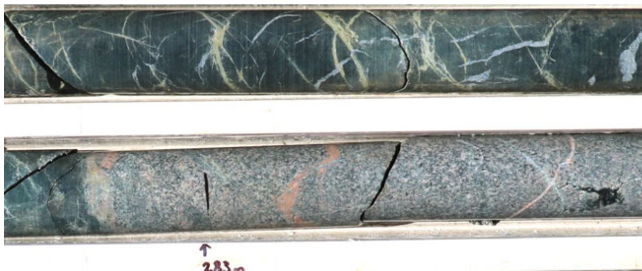
Figure 10 – AWN001 drill core at 282.1 metres (upper image) and 283.0 metres (lower image): 40 cm core lengths – Fine crystalline quartz- and feldspar-phyric quartz monzonite with pervasive potassic alteration, domainal actinolite and epidote alteration and stockwork fine quartz-albite-pyrite veins. Contact at 282.9 metres with strongly epidote-calcite altered magnetite-bearing basalt with stockwork calcite-quartz-epidote-pyrite veins.
