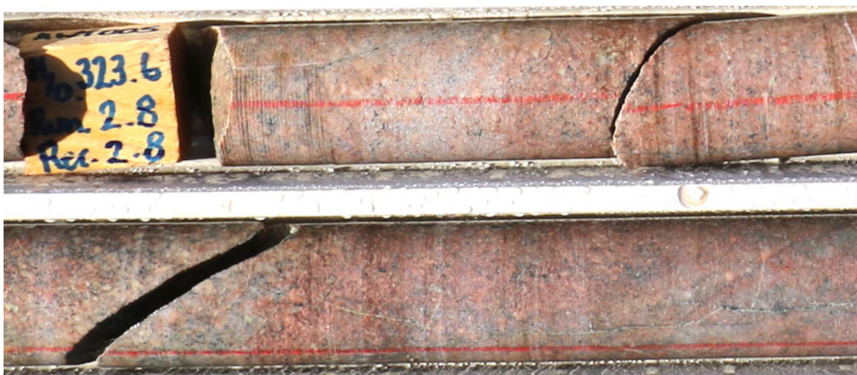
Figure 7 – AWT005 drill core at 323.6 metres (upper image) and 324.5 metres (lower image): 30 cm core lengths - Strong pervasive potassic altered feldspar-phyrlic syenite with fracture controlled chlorite alteration.
