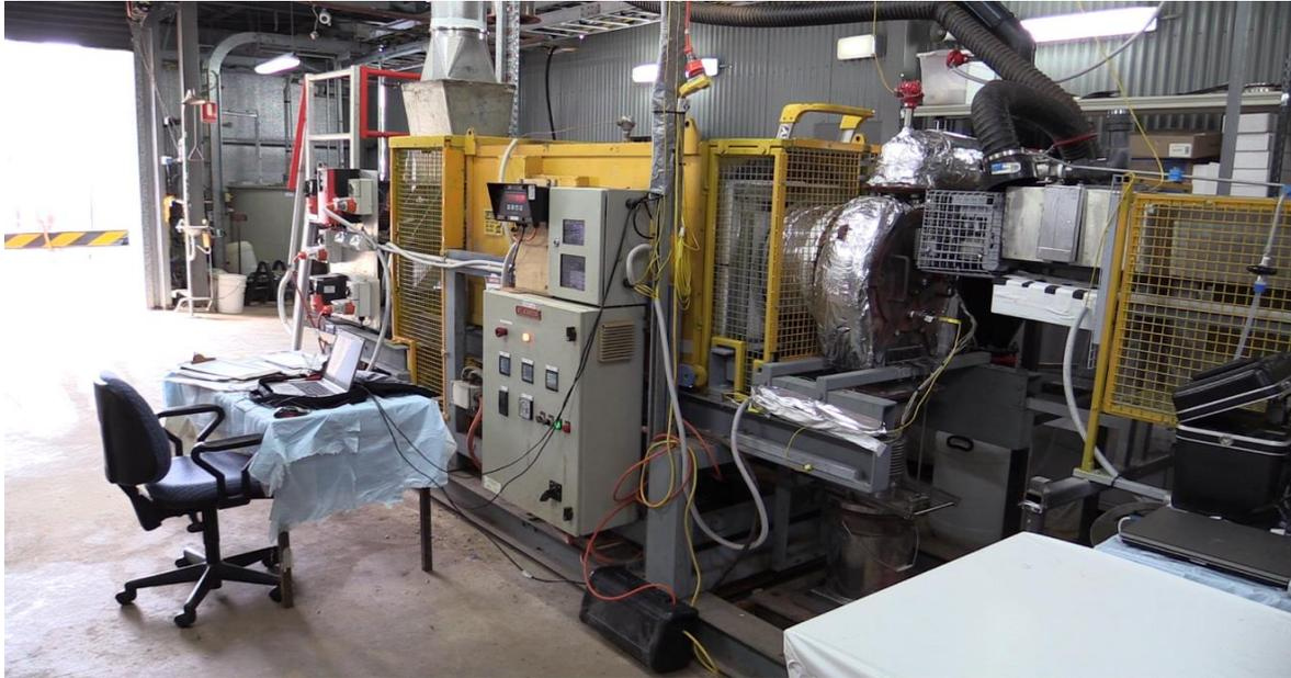
**Figure 2 Hydrometallurgical Pilot Testing - Acid Bake Kiln**
