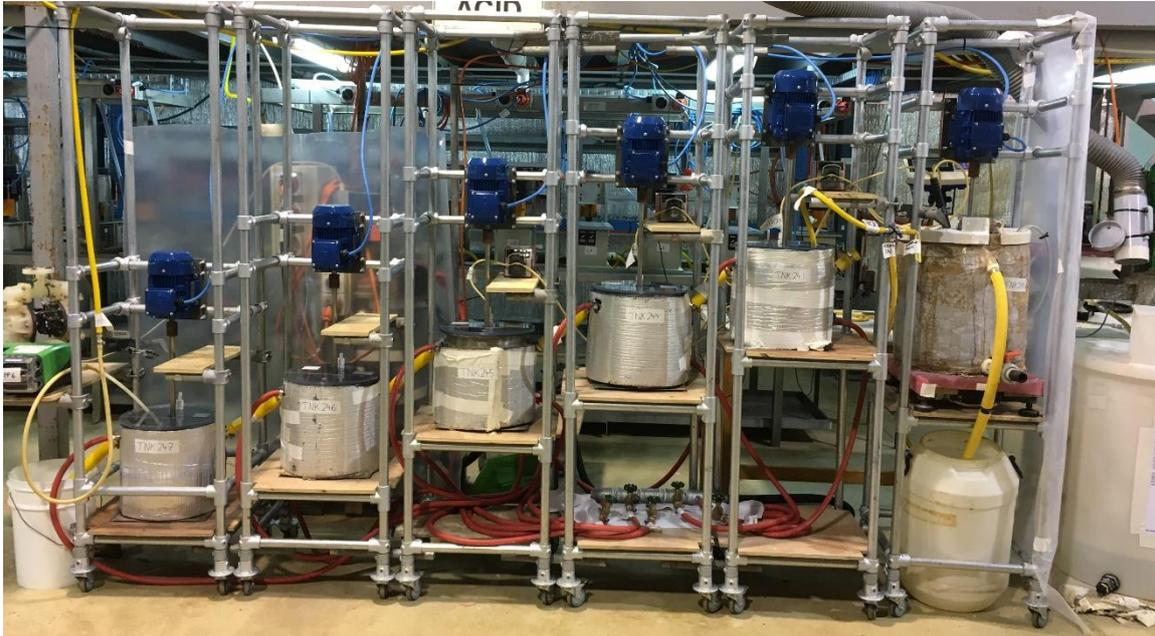
**Figure 4 Hydrometallurgical Pilot Testing – Neutralisation and Precipitation Circuit**
