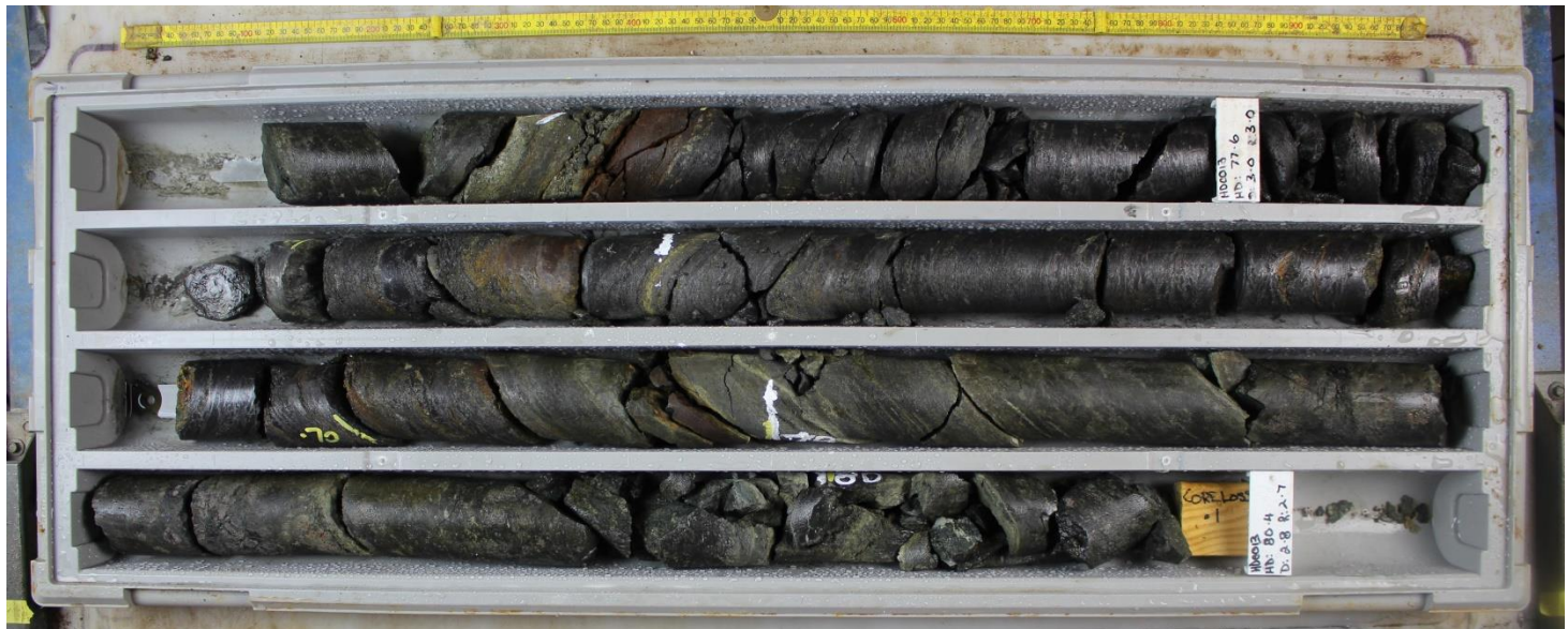
Figure 1. Diamond drilling graphite core from hole HD0013 (77 to 80.4 meters)
