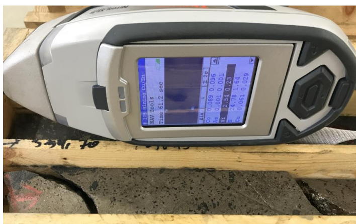
Pentlandite and pyrrhotite sulphide mineralisation with spot handheld XRF readings in LAI-08-034 (northern most drill line)
