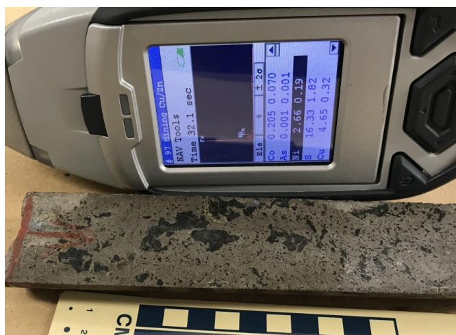
Pentlandite, pyrrhotite and chalcopryite sulphide mineralisation with spot handheld XRF readings in LAI-07-015
