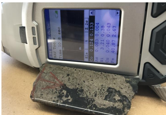
Pentlandite and pyrrhotite sulphide mineralisation with spot handheld XRF readings in LAI-07-015
