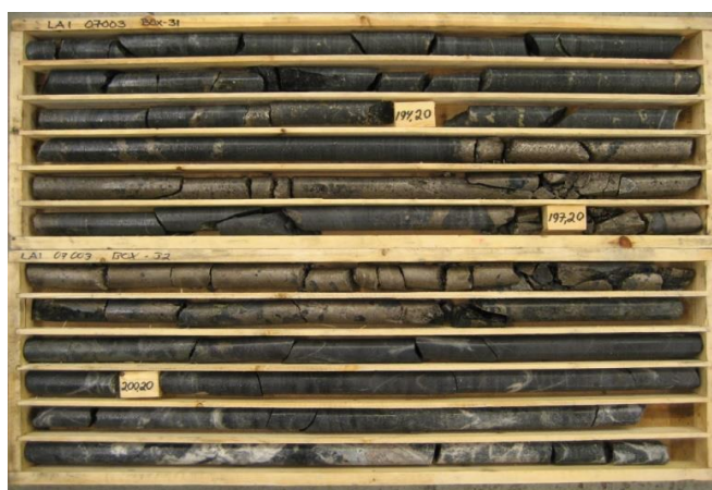
LAI-07-003 showing massive, pentlandite and chalcopryite and pyrrhotite mineralisation
