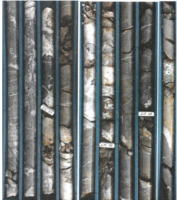
Figure 5 RIGHT Core tray photo showing the strongly mineralised vein HV-03/04 in RDDH-004.
