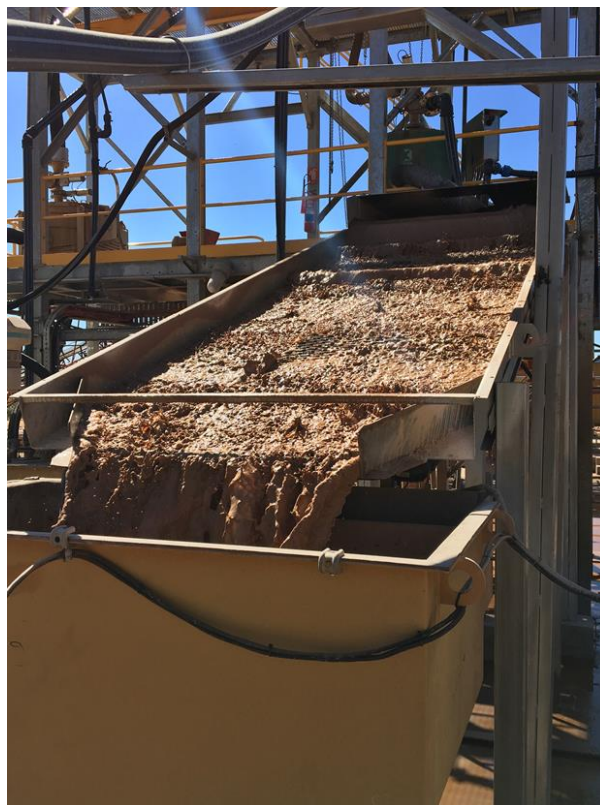
Picture 4: Sluice Box in operation
