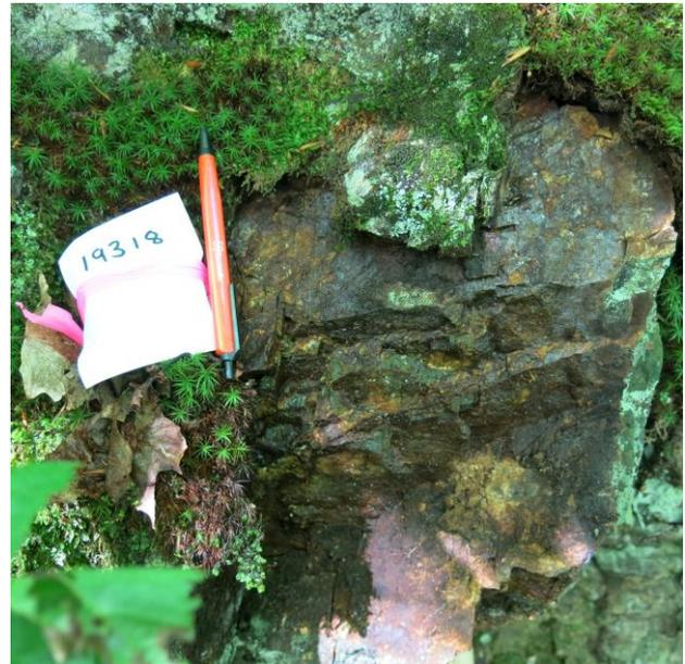
**Image 2:** Chalcopryrite and sulphides at surface in outcrops at the Lac du Marcheur cobalt project
