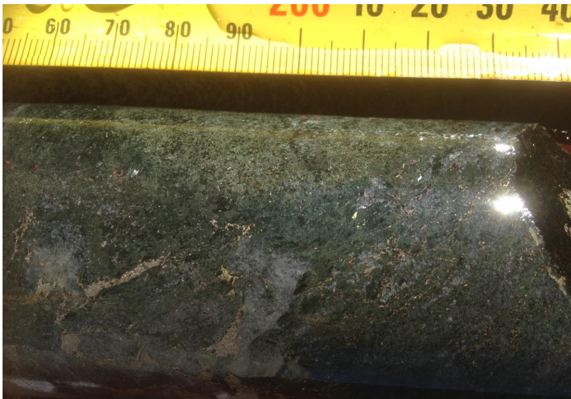
Image Four | Sulfides containing Nickel & Copper within the mafic-ultramafic gneiss at 219.7 metres down drill hole ODD01.
