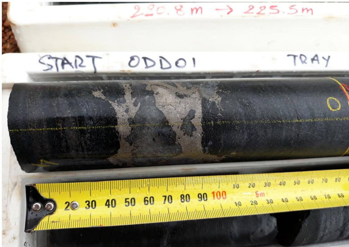
Image Three | Sulfides containing Nickel & Copper in the first drill hole at the Odin Prospect.
