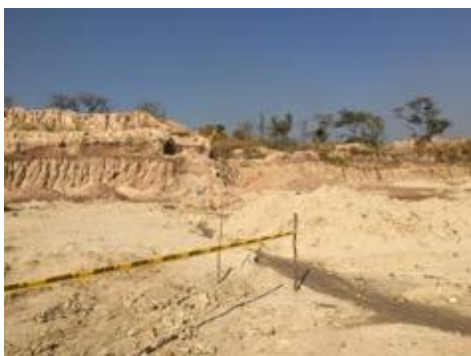
Images 5 and 6. Drill lines marked out in the Kania Main Pegmatite, the pegmatites exposed in the current main Kanuka mining area.
