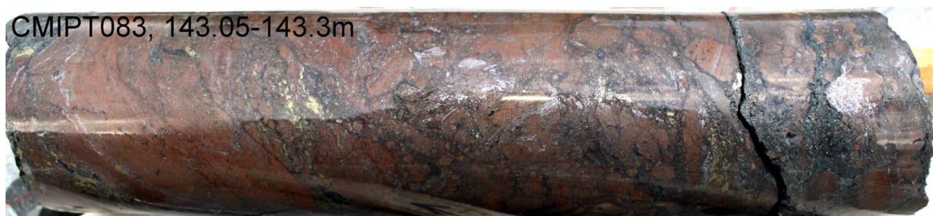
Figure 4. Hole CMIPT083: massive and brecciated massive sphalerite (red-brown) with lesser galena. Up to 3% chalcopyrite (yellow) is present in places.
