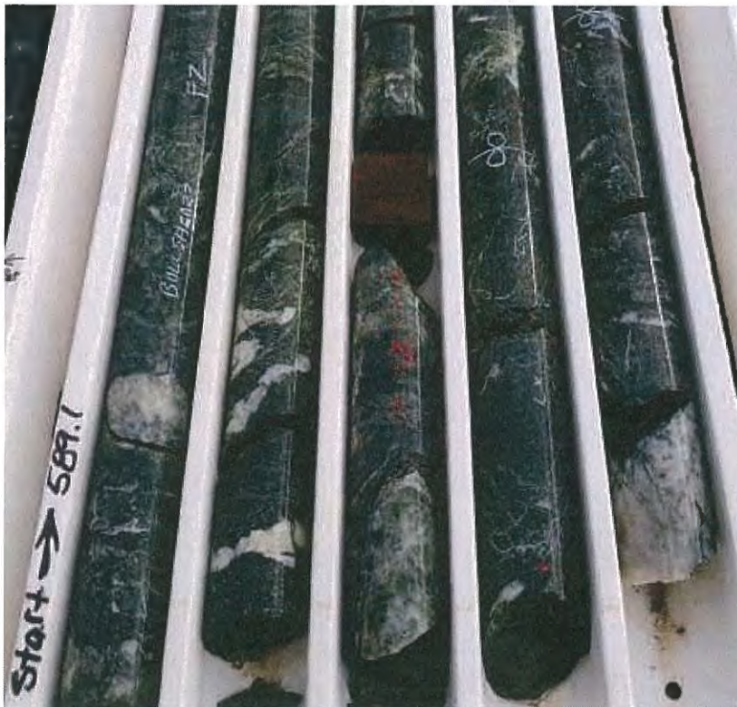
Figure . Photograph of strongly sheared drill core from FFD02, one of the holes at First Find
