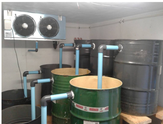
Chiller units for the evaporation / condensation process
