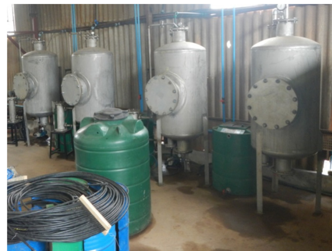
Evaporators and crystallisers (under vacuum)
