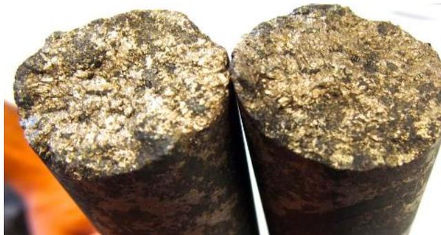
Image 1: Drill core from Mammoth showing Semi massive & veined mixed sulphides in sheared mafic host
