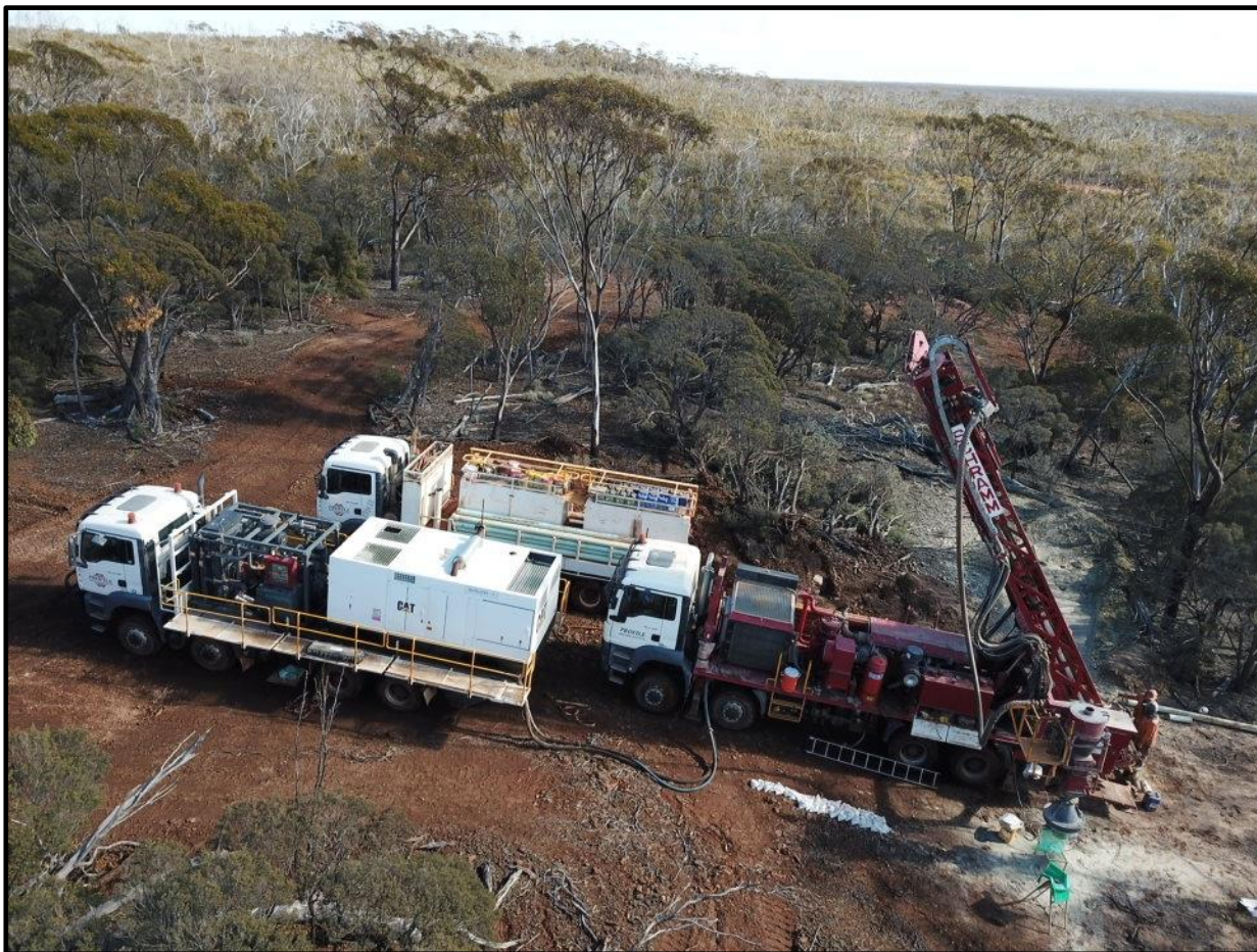
Figure 2: Buldania Project – RC drill rig at the Anna pegmatite
